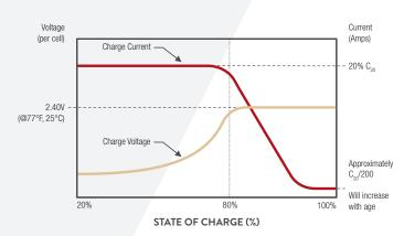
Note: Charging time will vary depending on battery size, charger output, and depth of discharge.
